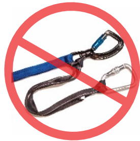
Figure 5: Do NOT create your own system that prevents the swivel from freely rotating during operation. This practice is not acceptable.
