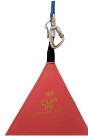
Figure 6: Attaching a belay gate to the swivel in such a way that it must be removed before climbing occurs is an acceptable solution to this problem so long as the swivel is never constrained during climbing, and such that connector stays with belay gate always. The belay gate must be attached using a carabiner with captive pin. With such a method, it must not be possible for climber to remove the second connector from the belay gate.
