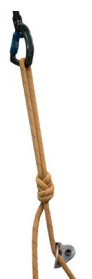
Figure 4: If attaching a tagline, attach directly to a carabiner in such that it is not constraining the swivel, and must be removed before connecting, as shown.
