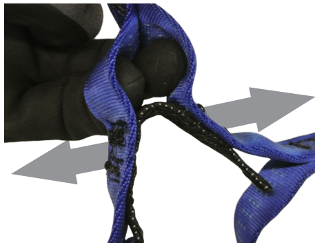
Activation Strip Inspection
