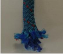
*Frayed ends must be properly terminated*
