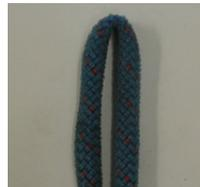
*If the rope kinks, the core has been compromised & must be retired*
