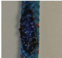
*Ropes with burns or signs of high heat exposure must be retired*
