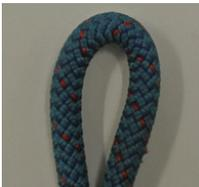
*When looped, the rope must hold a circular shape*
