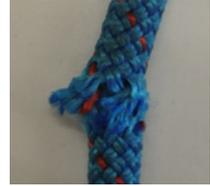
*Nicked or cut rope must be retired*
