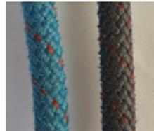
*Discoloration from Gorilla Rope running through pulleys and standard use is to be expected and is OK. Be sure to continue to inspect rope daily.*
